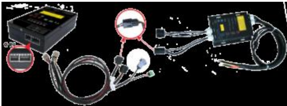
Figure 2-27 Example Diagram for Connection of Communication Cables between LDM and BCU
