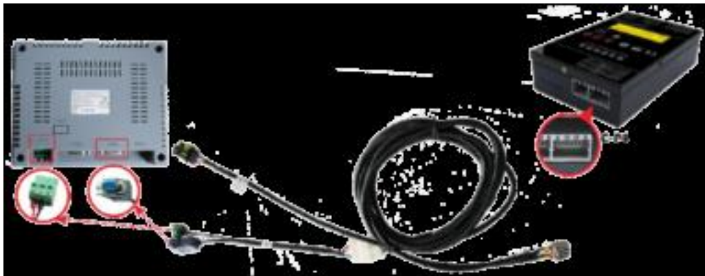
Figure 2-29 Example Diagram for Connection of LCD and BCU (take 5.7" one for example)
