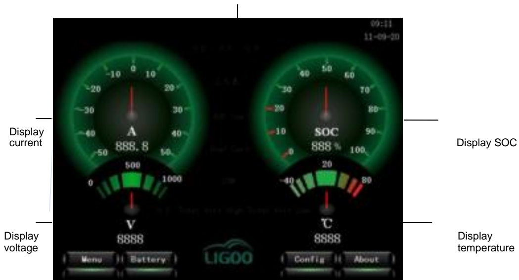
Figure 4-1 Main Interface of Terminal User
